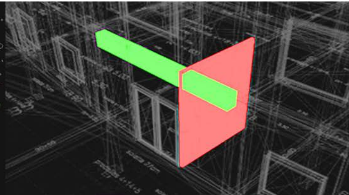
CLASH DETECTION: ARCHITECTURAL- STRUCTURAL-MEP
